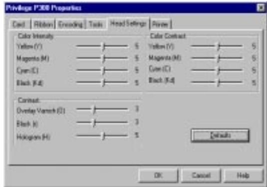
**Color Intensity** - Sets the values of yellow, magenta and cyan, and dye diffusion to adjust the amount of heat applied, to transfer a maximum intensity color or monochrome dot.
