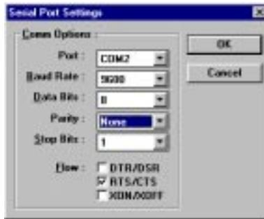
4. Select the port your PDF card reader uses (normally COM2). Check the correct baud rate and data format of your computer system. See your PDF Card Reader manual for the correct settings. **Click OK** to confirm your settings.
