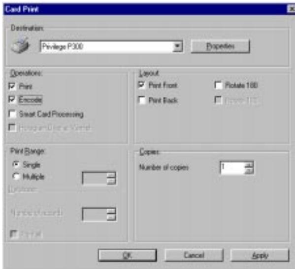
8. Select the **Encode** check box to enable magnetic stripe encoding.
