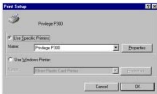
2. Check **Use Specific Printer** and select your printer type name. Click Properties. The specific printer dialog box appears. *Click* the ribbon tab.
