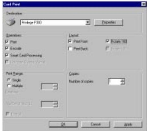
2. Select the Destination corresponding to the installed card printer. Use the properties button to change the selected printer configuration. Destination may be specific printers any printer through Windows driver or the print manager (printing to a batch file).
