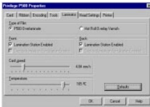
You can Laminate your card either with Varnish or with P500 Overlamine, check the type of film you will be using for the lamination process.
